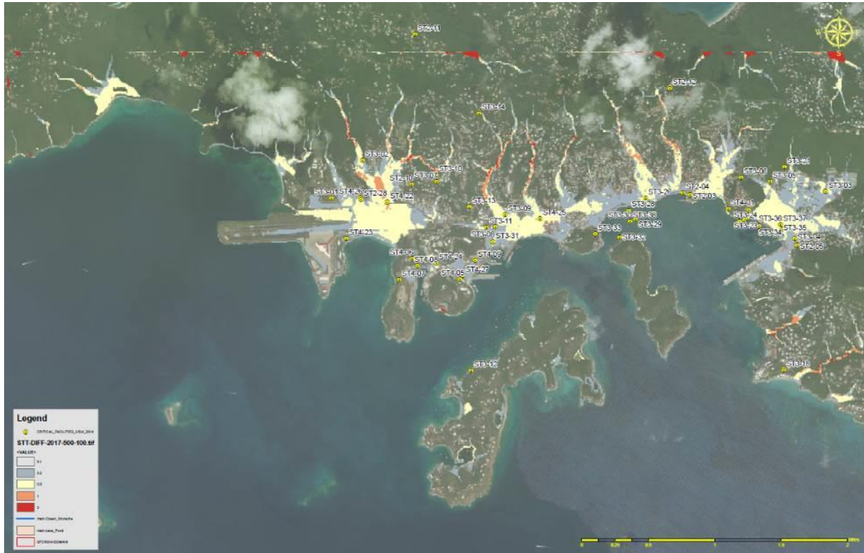
Figure 4.3: Difference in Flood Depths for a 100-year 72-hour storm event for year 2100 using the baseline intensity and the projected 30% increase. The aerial shows the topography and difference of computed depths of water
