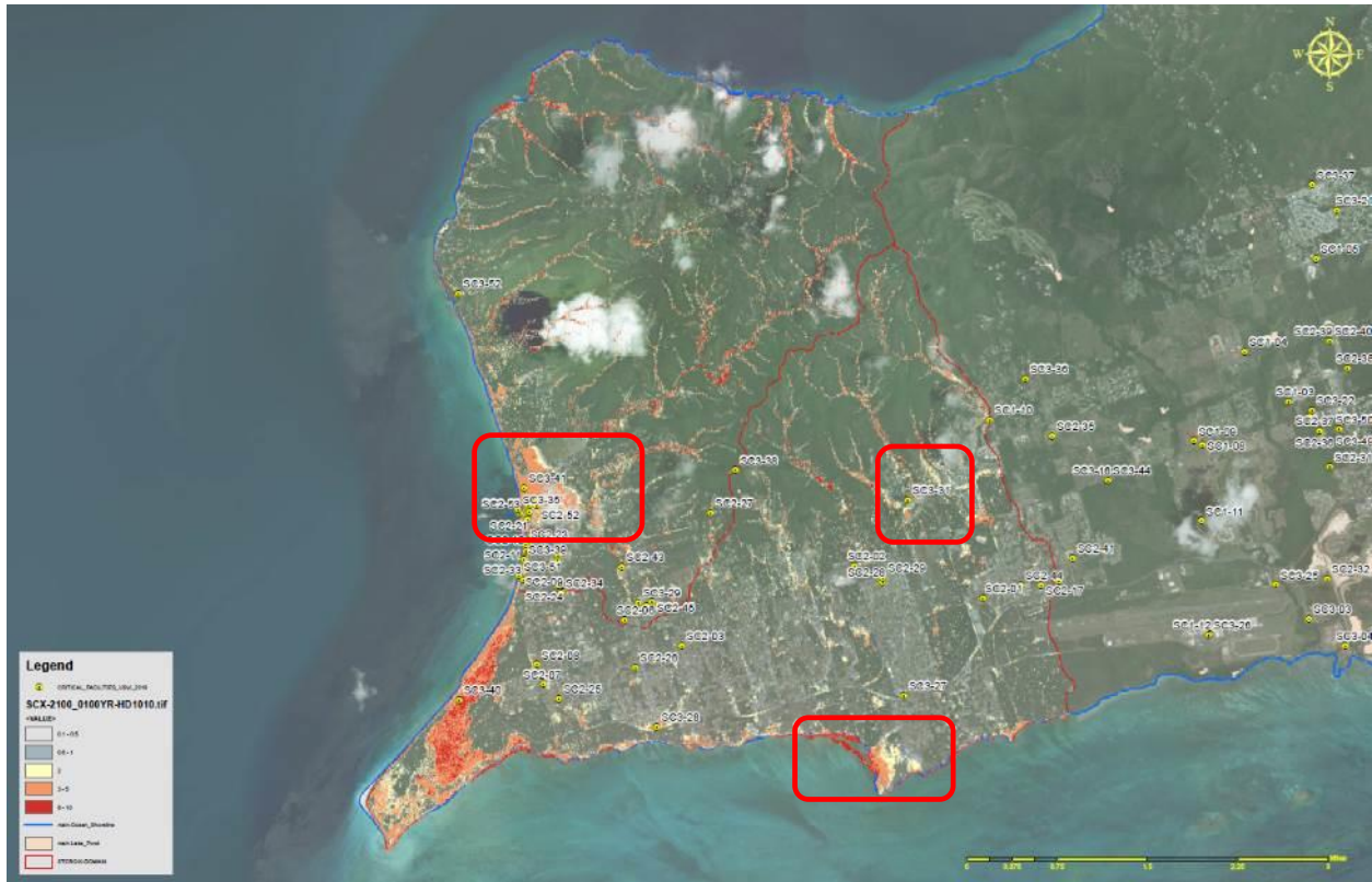
Figure 6.21: Flood Depth Analysis of 500-year 72-hour storm event for year 2100. The aerial shows the topography and computed depth of water (Appendix A14.MAP_STT_2065_0500_HD.pdf provides a higher resolution map).
