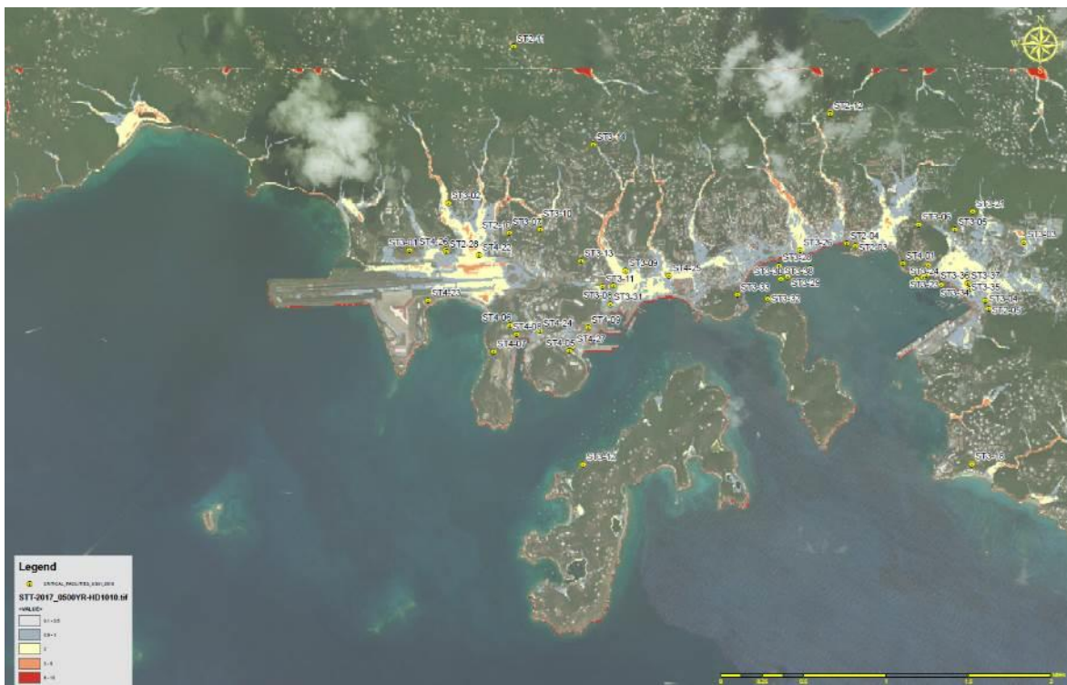
Figure 6.18: Flood Depth Analysis of 500-year 72-hour storm event for year 2100. The aerial shows the topography and computed depth of water and areas of concern where flood depth greater than 2 ft is observed (Appendix A14.MAP_STT_2065_0500_HD.pdf provides a higher resolution map).
