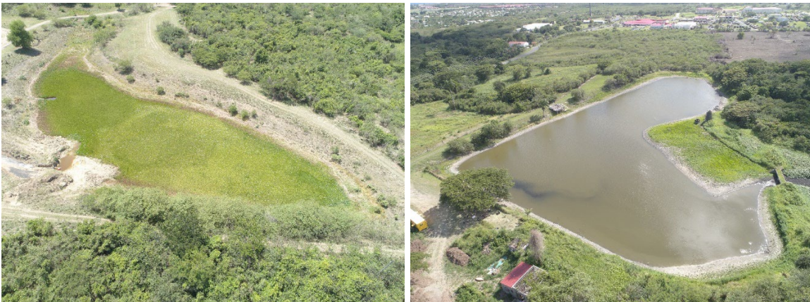
Figure 2: VIDA water ponds on St. Croix showing sediment accumulation that need to be dredged – Photo by VI Aerial in July 2021.
